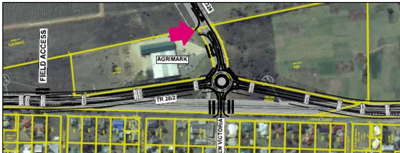
Figure 5: The proposed traffic circle at Stanford.
