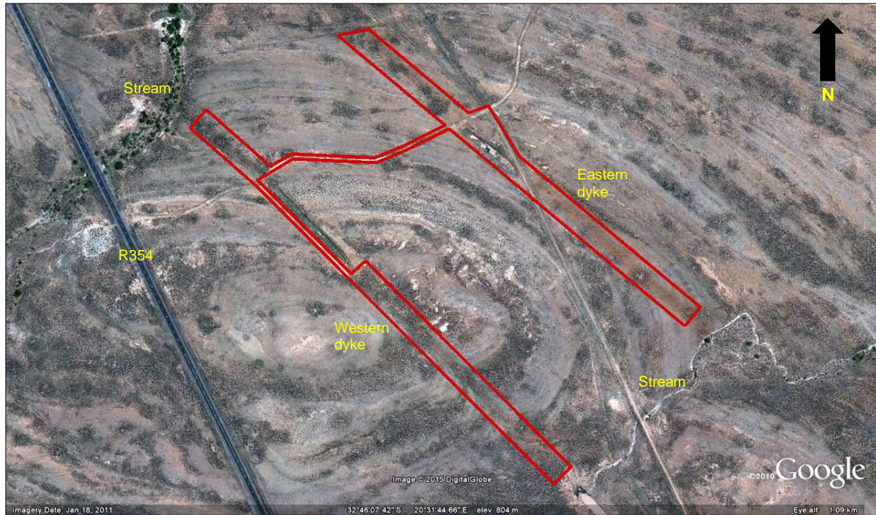
Figure 4. Google satellite map illustrating the proposed application area for the Karusa R354 borrow pit.
