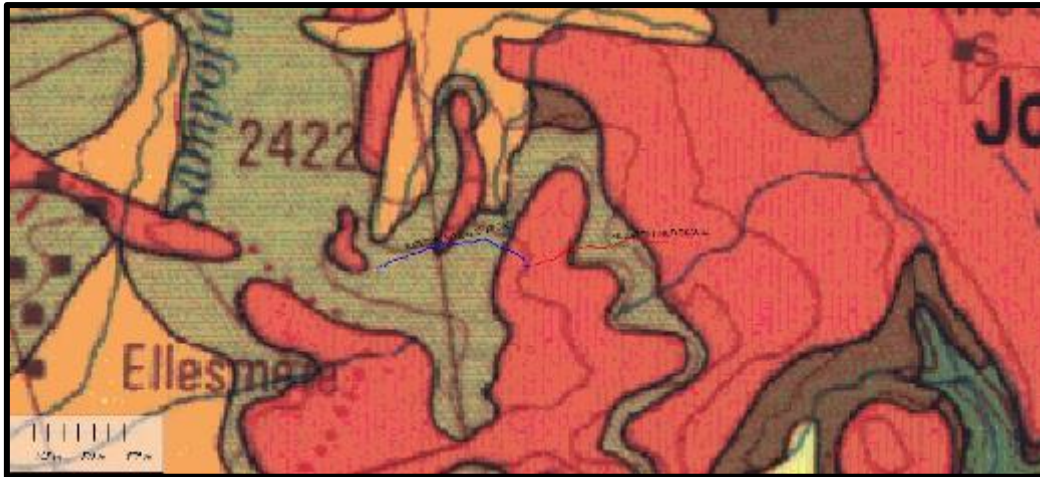
Figure 3 Geology of the Mthaleni 2 Ext Road Area. Vryheid Formation (Pv; grey) and dolerite (Jdo; pink) sills.
