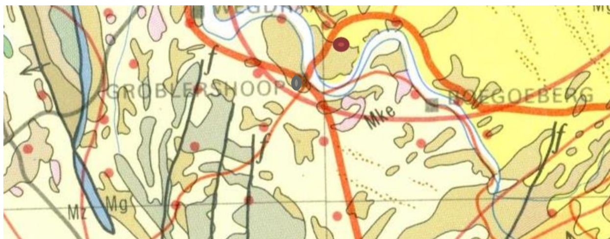
Figure 12: Extract of the 1:250 000 geological map of the Groblershoop indicating the approximate position of the proposed development (indicated in blue), on portion 17 of farm Boegoeberg settlement number 48, !Kheis Local Municipality in the Northern Cape Province. The development is underlain by the Groblershoop Formation.
