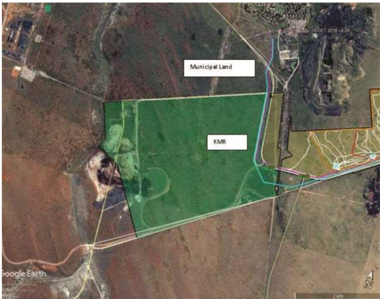
Figure 9: The route of the proposed 132 kV powerline, from York A 279, across the railway line and R31, through the property of KMR and Municipal land, connecting with the Hotazel substation, a distance of 6km in total.
