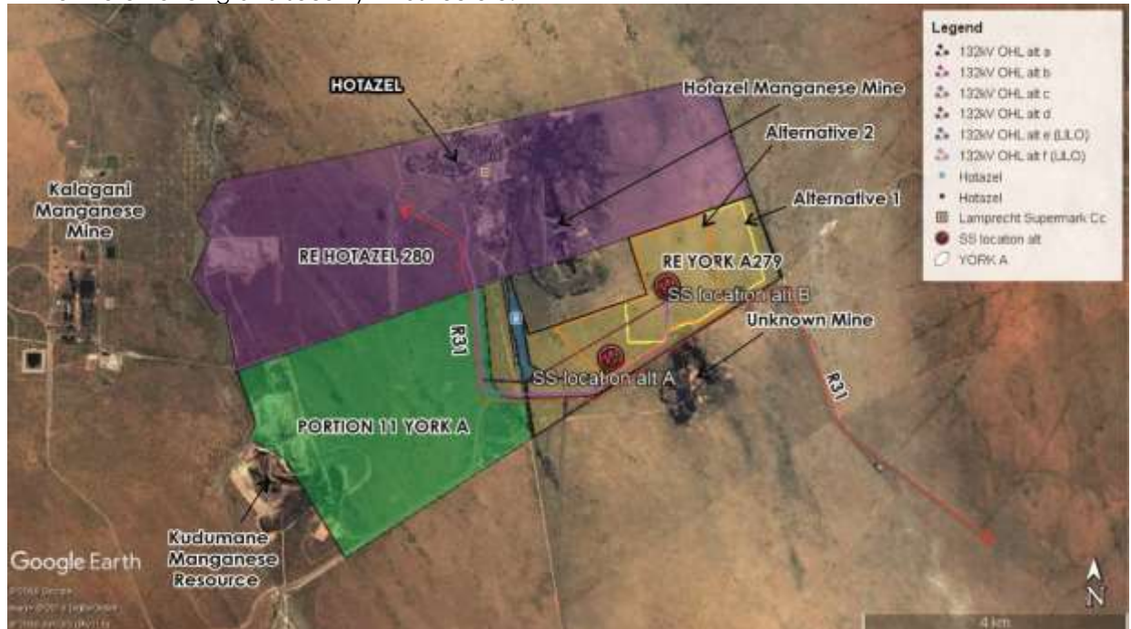
Figure 4: Location of the two alternative on-sit substations are shown as Alt A and Alt B. Alternative 2 is the preferred option (Source: Google Earth, 2018).
