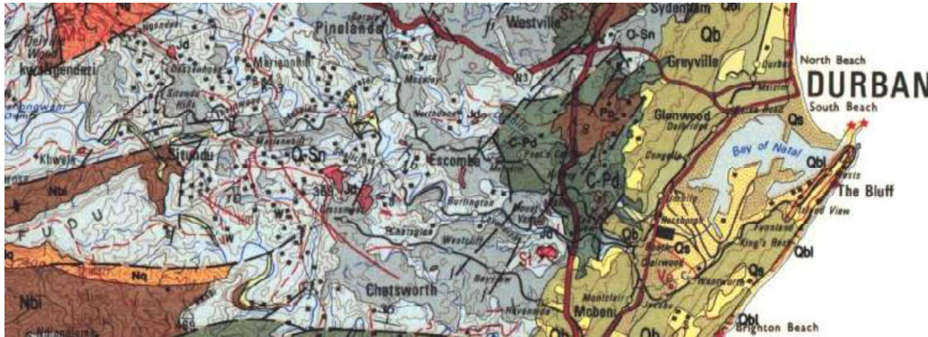
Figure 2: Approximate area of the proposed Housing Development on ERF 1359, Queensburgh, 35-53, Huntley Road, eThekweni, KwaZulu-Natal. Extract from the 125 000 Geological Map: Durban 2930. According to this map this project will intersect the Natal Group (grey) and possibly Karoo Dolerite (Jd: red).
