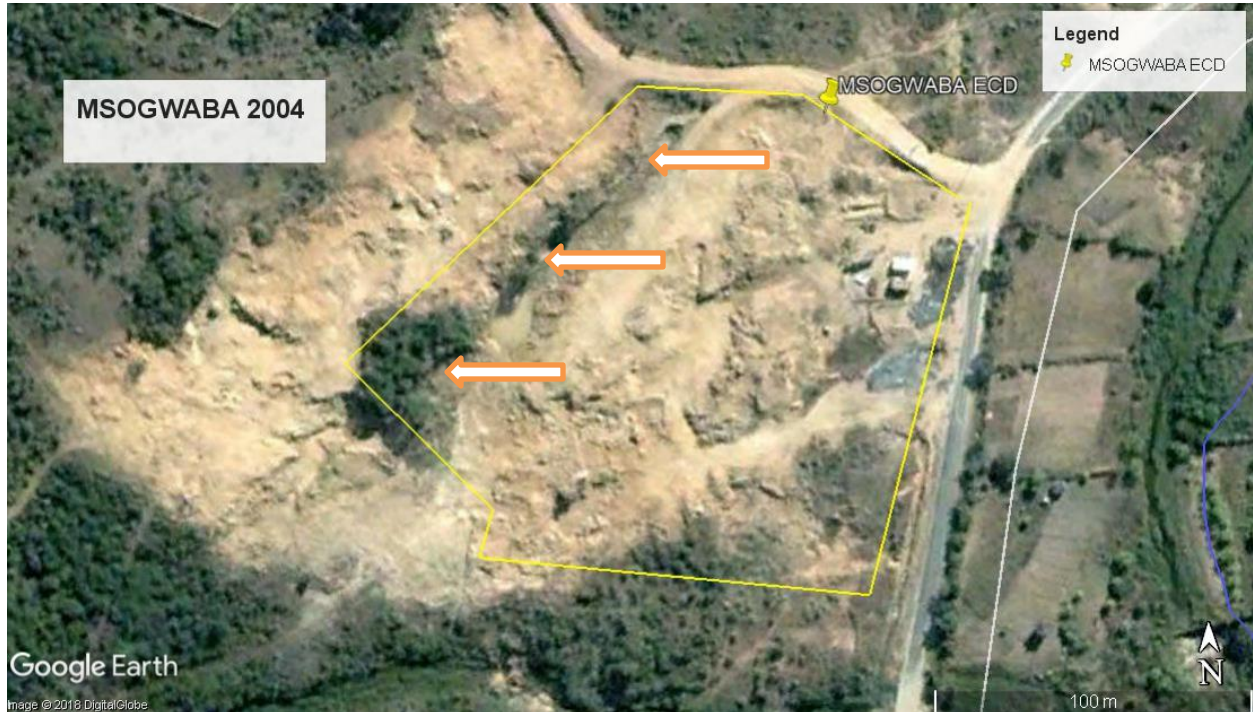
MAP 8: The 2004 image of the study area (yellow line) show the extent of the disturbance. The entire area was extensively used as a borrow pit until granitic / sandstone bedrock was reached. The area where the rocky ridge is, is visible at the western border (see arrows).
