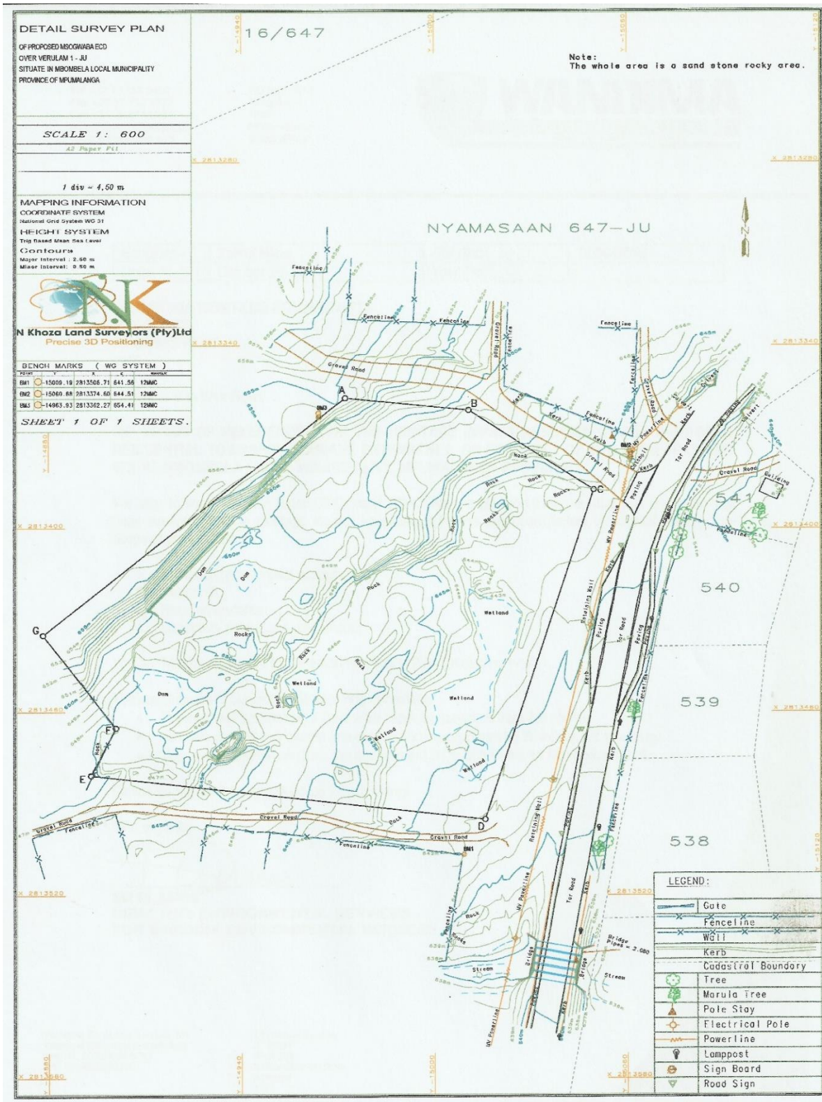
MAP 2: Detailed surveyors plan of the Msogwaba YDC, (N. Khoza Land Surveyors (Pty) Ltd.). Please note the exposed sandstone rock surface, wetlands and dams, indicated on the map.
