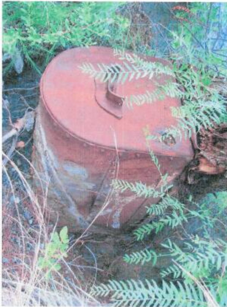
Figure 361: An old cocopan lying on its side. These narrow ones predate the ones that flare out towards the top as in the example below
