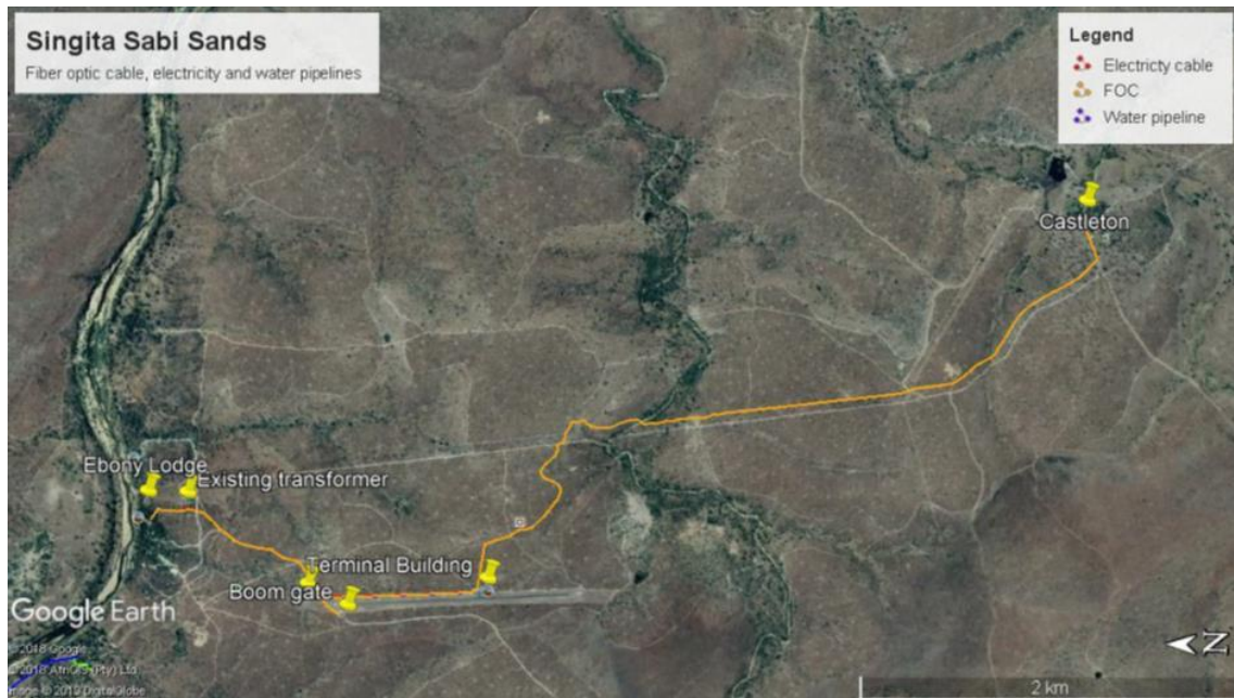
FIGURE 23 THE ROUTE OF THE FIBRE OPTIC CABLE FROM CASTLETON TO EBONY LODGE VIA THE TERMINAL BUILDING (Taken from Zunckel 2019).
