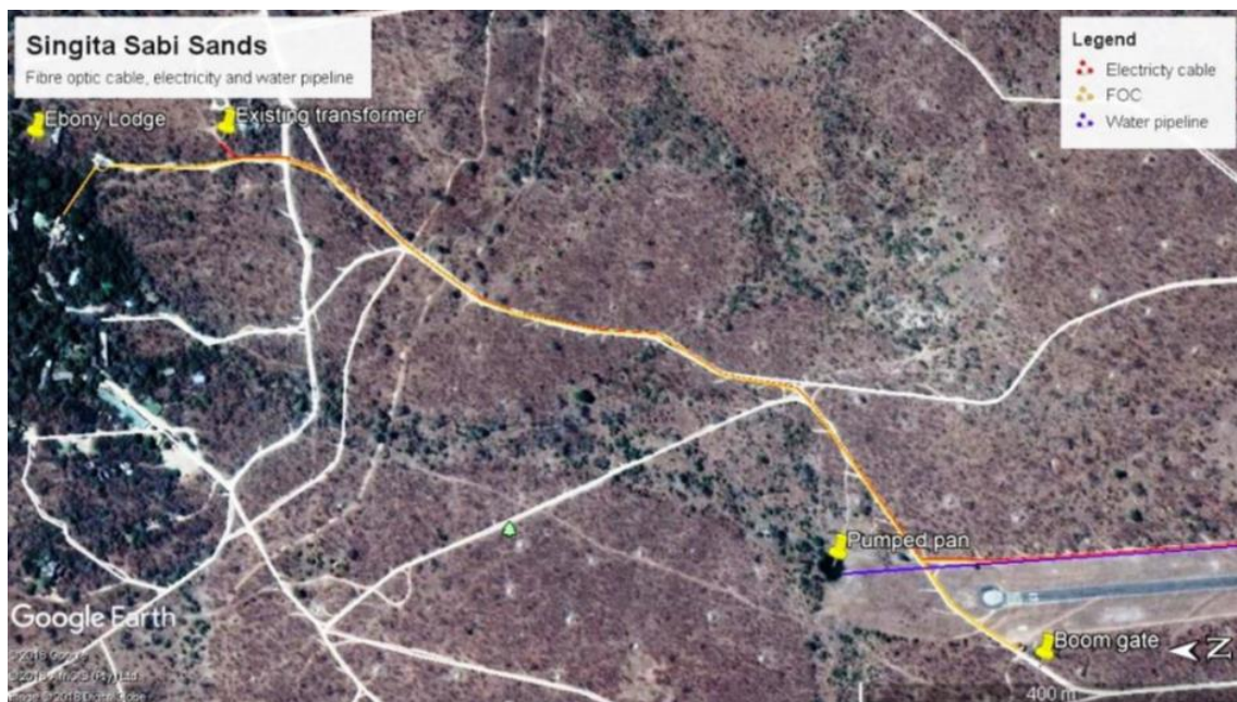
FIGURE 24: ZOOM INTO THE FOC ROUTE TO EBONY LODGE SHOWING THE ELECTRICITY CABLE FROM AN EXISTING TRANSFORMER TO THE TERMINAL BUILDING (RED) AND THE WATER PIPELINE FROM THE PUMPED PAN TO THE TERNIMAL BUILDING (BLUE) (Taken from Zunckel 2019).
