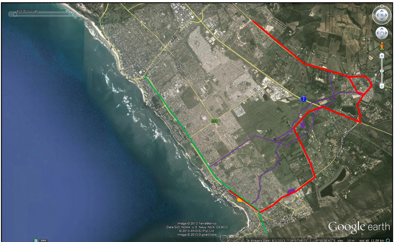
Figure 1: The proposed fibre optic duct route is shown in red. The Gordon's Bay Midden is shown as a yellow polygon. The areas to the west of the green line are identified by the city as archaeologically "sensitive". The purple polygons and purple lines indicate properties and routes previously assessed for archaeology.
