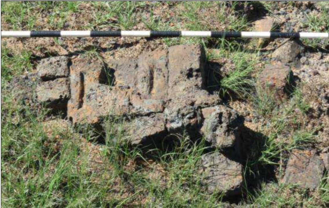
Figure 14 – One of the brick mounds from the lower end of the site. It is evident from this photograph that the bricks were fused together during the brick making process. The effects of extreme heat during the firing process can clearly be seen on these bricks.
