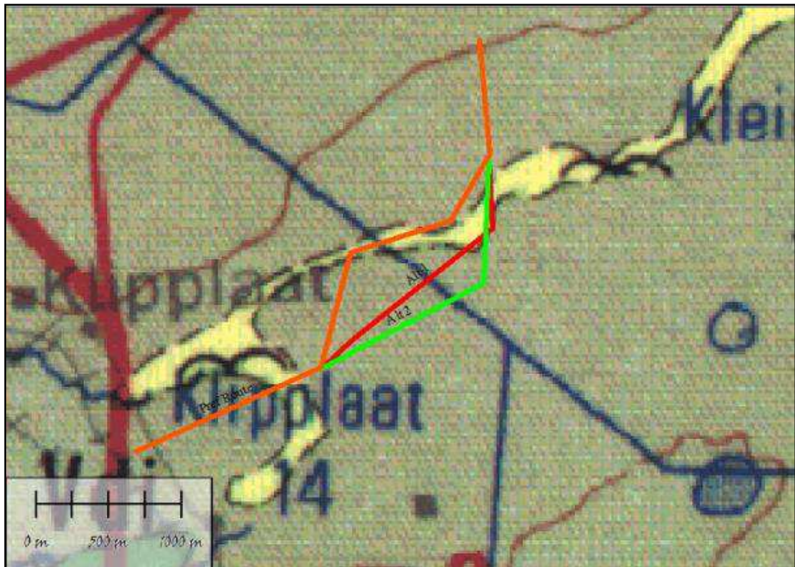
Figure 23 – Overlay of the three development alternatives relative to the geology of the area.
