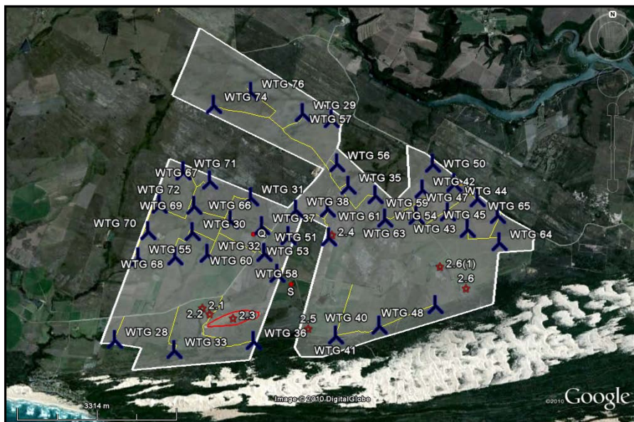
Figure 23: Final development design of the Central Cluster study site indicating turbine positions with final numbering and access roads (yellow) in relation to the Phase 1 AIA assessment area and identified site localities (red stars) and site boundaries (red outline)
