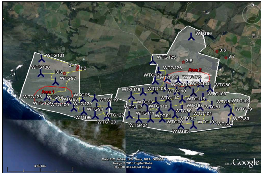
Figure 45: Final development design of the Western Cluster study site indicating turbine positions with final numbering and access roads (yellow) in relation to the Phase 1 AIA assessment area and identified site localities (red stars) and site boundaries (red outline)
