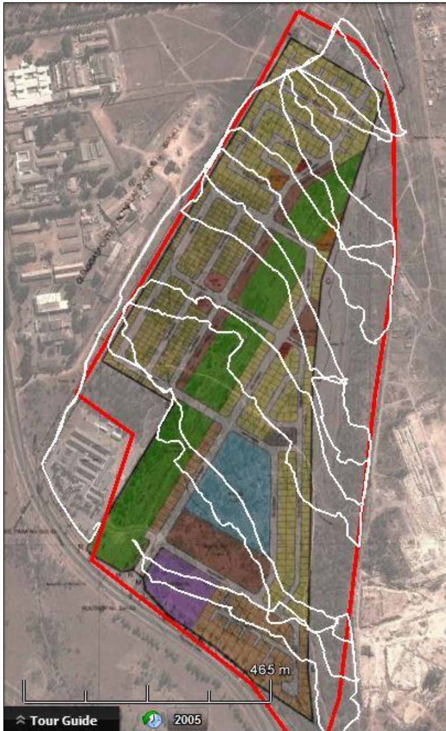
Figure 20 – Google Earth map depicting the following elements: the study area boundaries that were provided by the client (red line), the recorded track logs (white line) and finally the actual development layout plan shown as an overlay.
