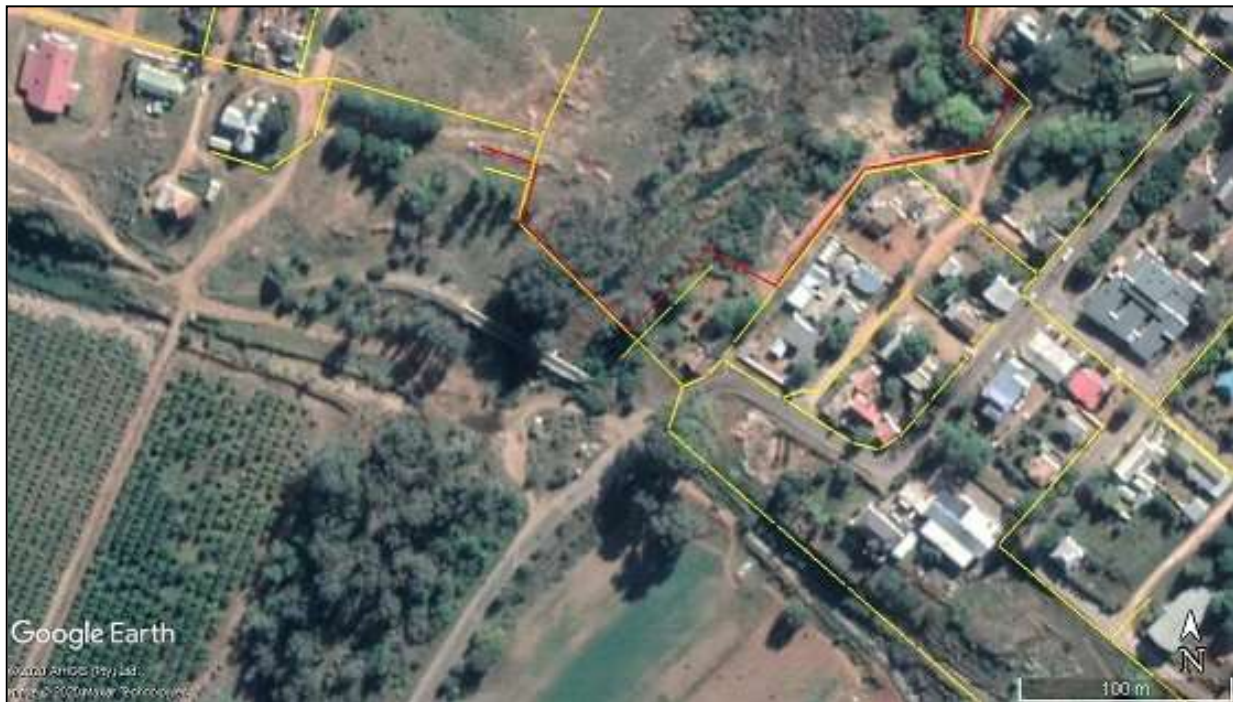
Map 7. Aerial views of the location of alternative option 2 (red line) and alternative option 3 (yellow line) for the sewer pipeline crossing the Klein River
