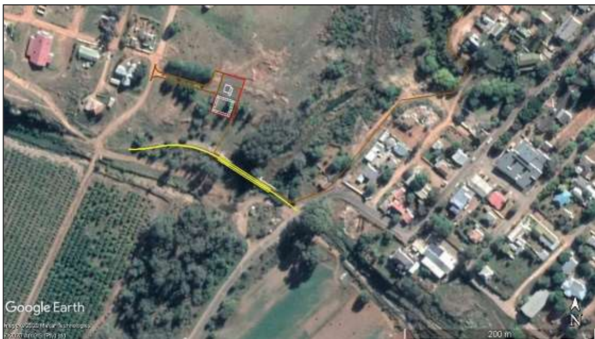
Map 6. Aerial view of the location of the preferred option of the sewer pipeline crossing the Klein River by installing the pipeline on the existing “Narrow Gauge” Steel Rail Bridge indicated in yellow. The pipeline is indicated by the light brown lines. The access road is indicated by the dark brown lines (also see Map 3) and the pump station and detention pond by the white squares.
