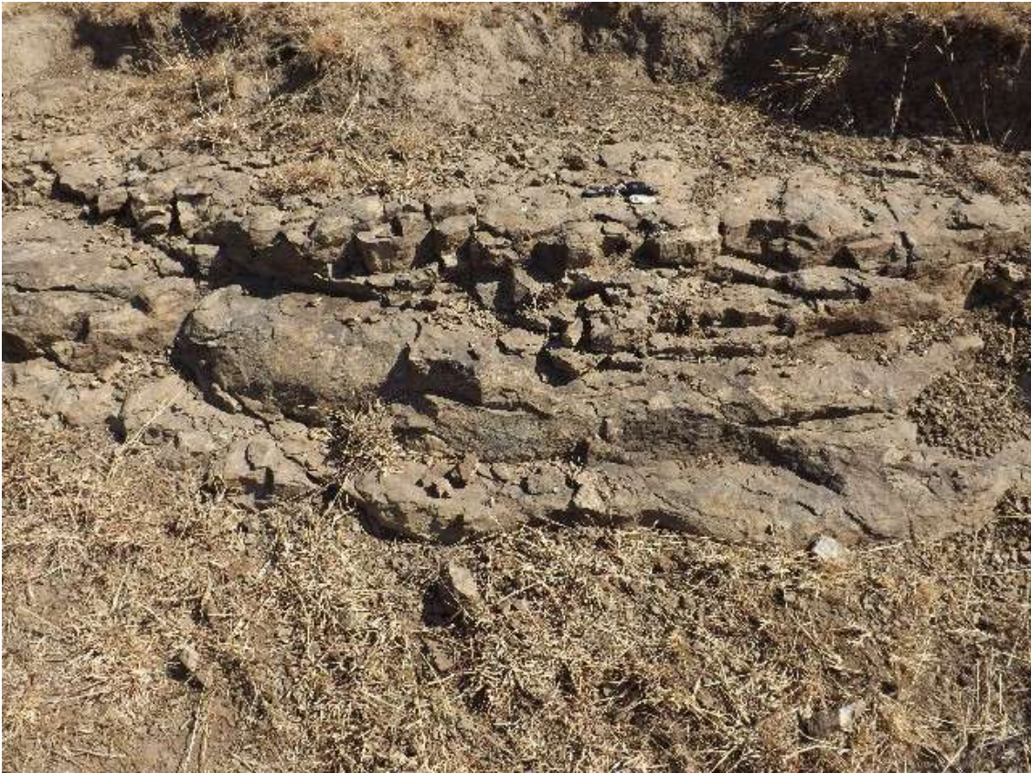
Figure 4: An example of the Estcourt Formation as it could occur in the proposed development area. However this lithology is expected to be deeply weathered on this site, but there could be fresh rock at depth (>2m).
