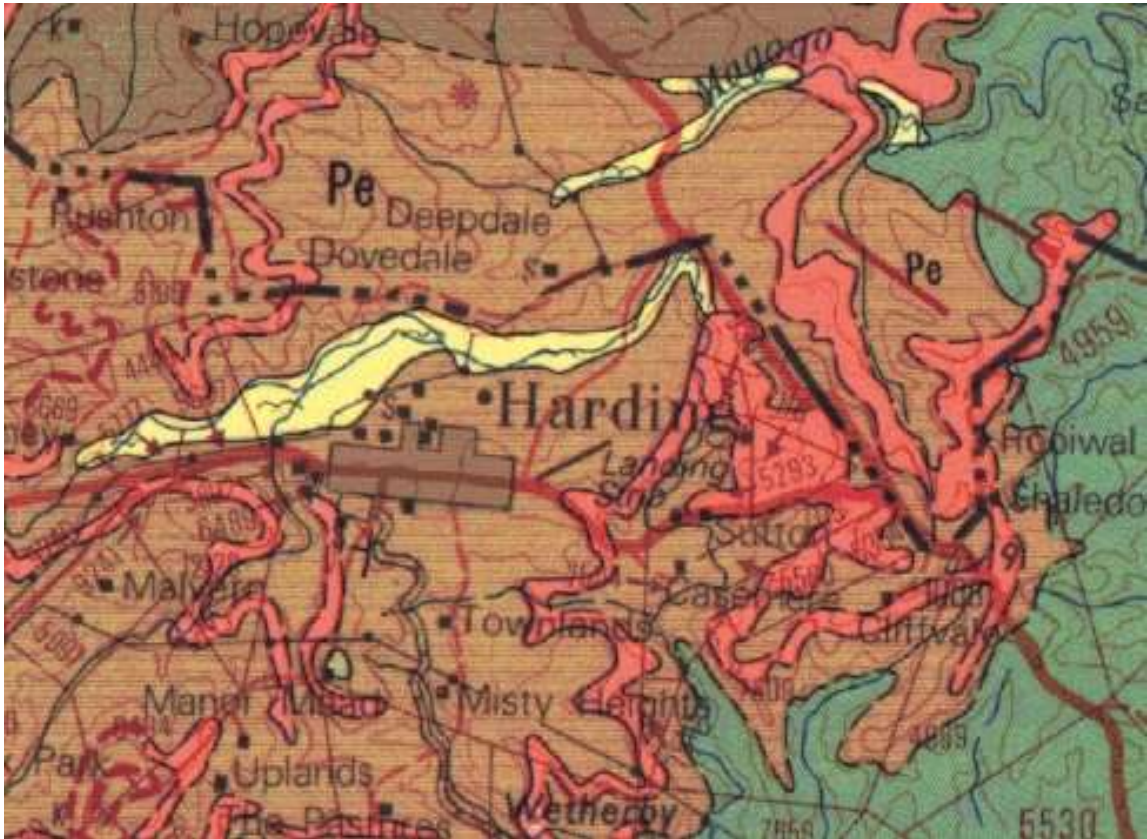
Figure 3: Extract from the Kokstad (3038) 1: 250 000 Geological Map. Grey (Pa) is the Estcourt Formation and red is Karoo Dolerite.
