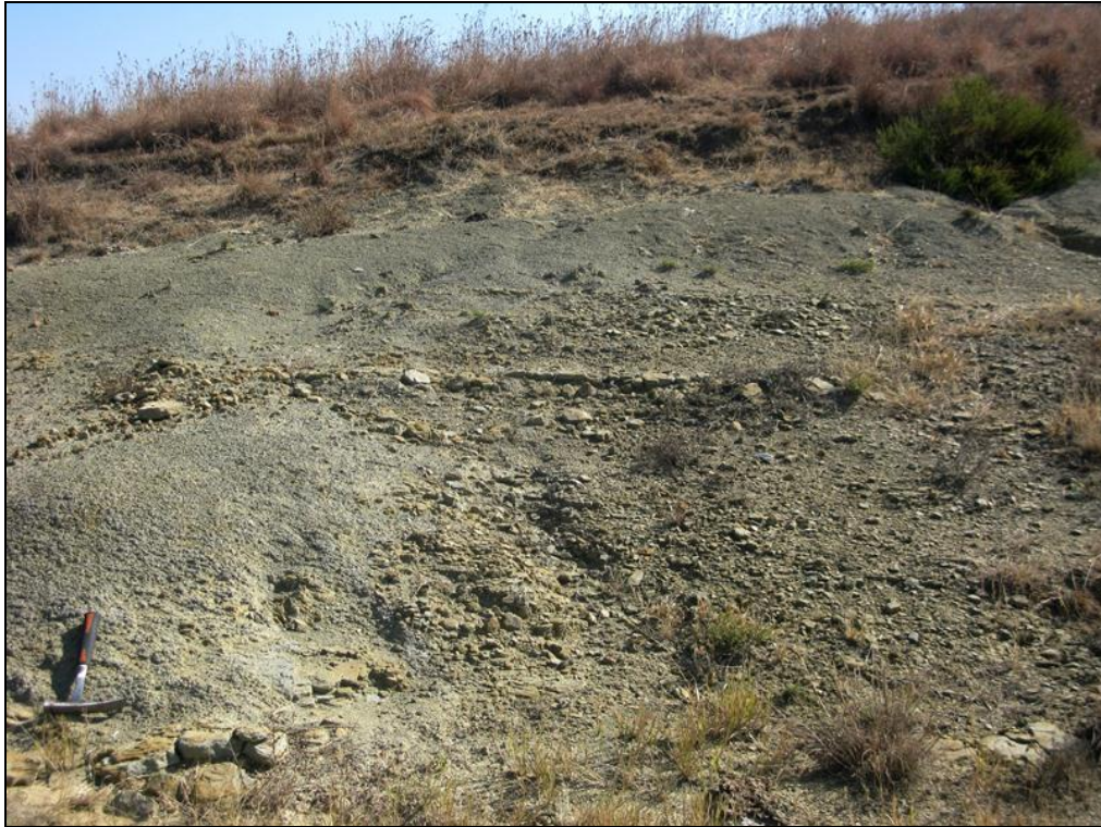
Figure 19. Hillslope exposure of grey-green expansive-weathering mudrocks and thin sandstone interbeds along the west bank of the Rietspruit (Loc. 283) (Hammer = 30 cm).
