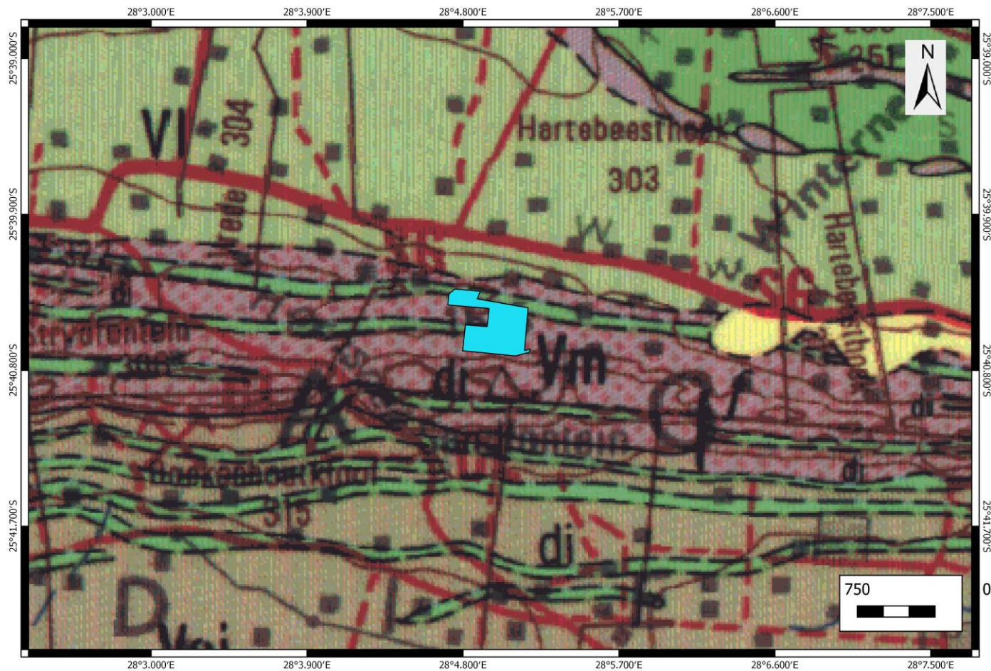
Figure 5: Extract of the 1: 250 000 2528 Pretoria Geological map (Council of Geoscience) of the proposed Residential development in Gauteng. (development footprint indicated in blue). The proposed Residential development in Gauteng is primarily underlain by the Magaliesberg Formation of the Pretoria Group (Transvaal Supergroup). Map drawn by QGIS 2.18.28.
