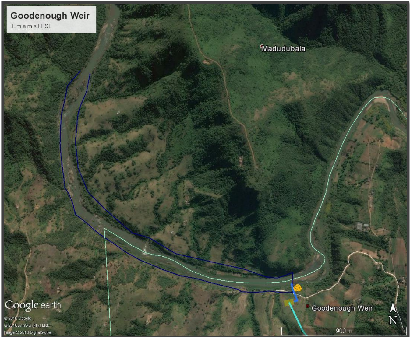
Figure 3 Approximate FSL of raised Goodenough Weir (30 m a.m.s.l)
