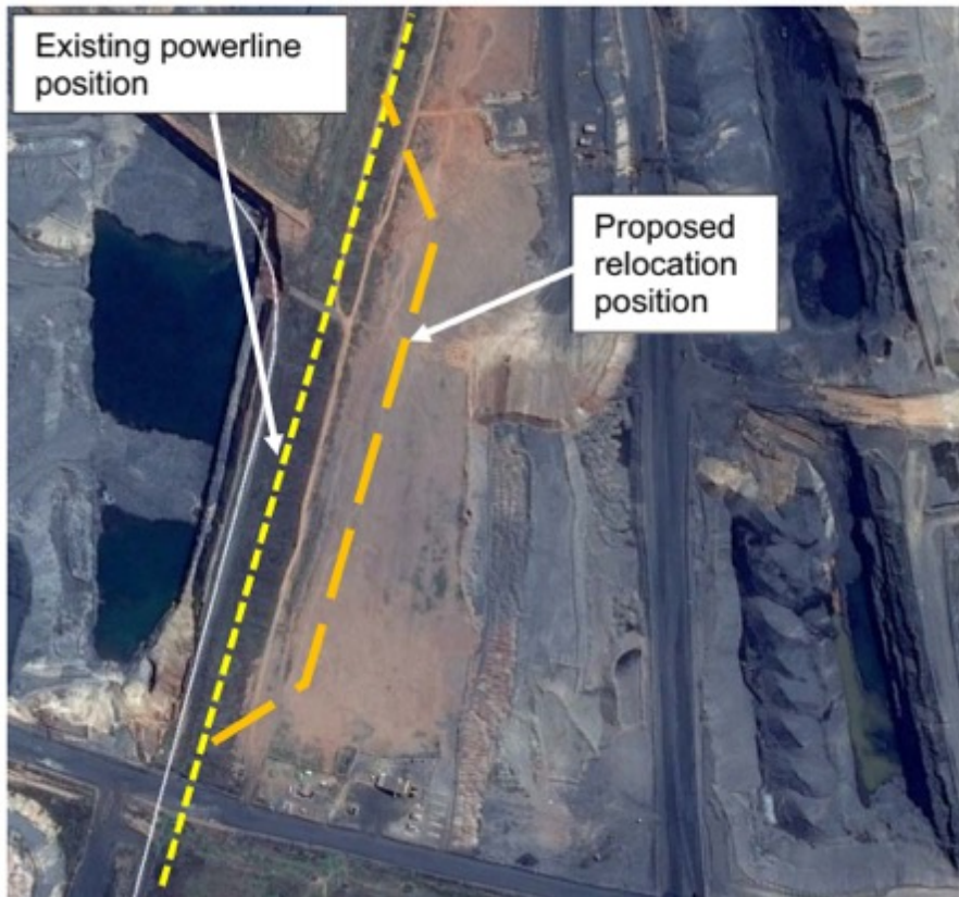
Figure 3: Proposed position of the deviated lines. Also note the disturbance of the landscape.
