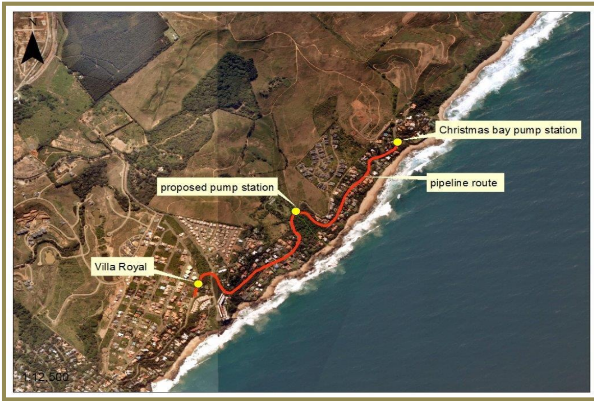
Figure 2 Aerial View Sewer Line Route
