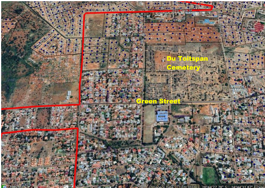
Figure 33: Kirstenhof area of Route 2. The red lines shows that the area falls within the older than 60 years area. The blue dots show the position of the poles for the aerial fibre
