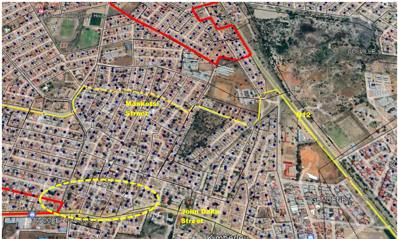
Figure 25: Section 5 of Route 1 (Galeshewe): Yellow line indicates the underground main line and the blue dots the position of the poles for the aerial fibre. The red lines show the boundary of the area older than 60 years. The dotted lines show the block within Greater nr 2 area containing most heritage significance in this area.
