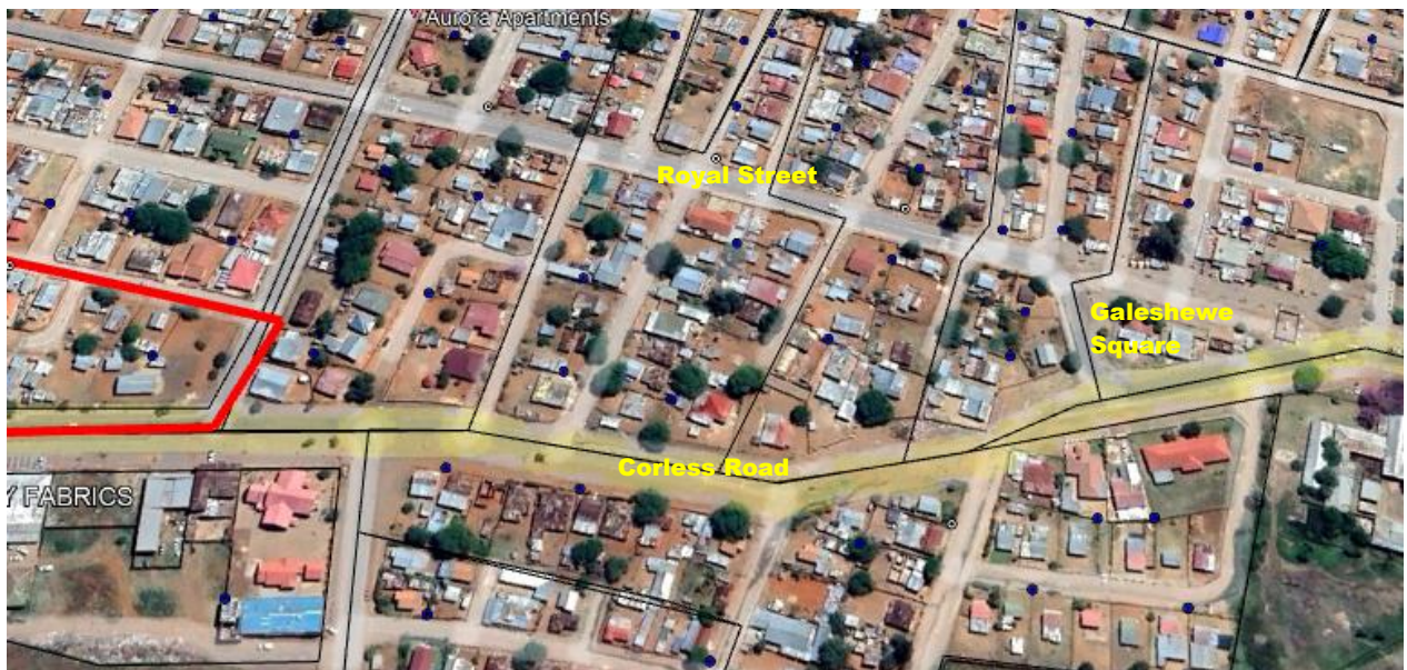
Figure 26: Street block between Royal Street and Corless Road. Blue dots show the position of the proposed mid-block aerial fibre
