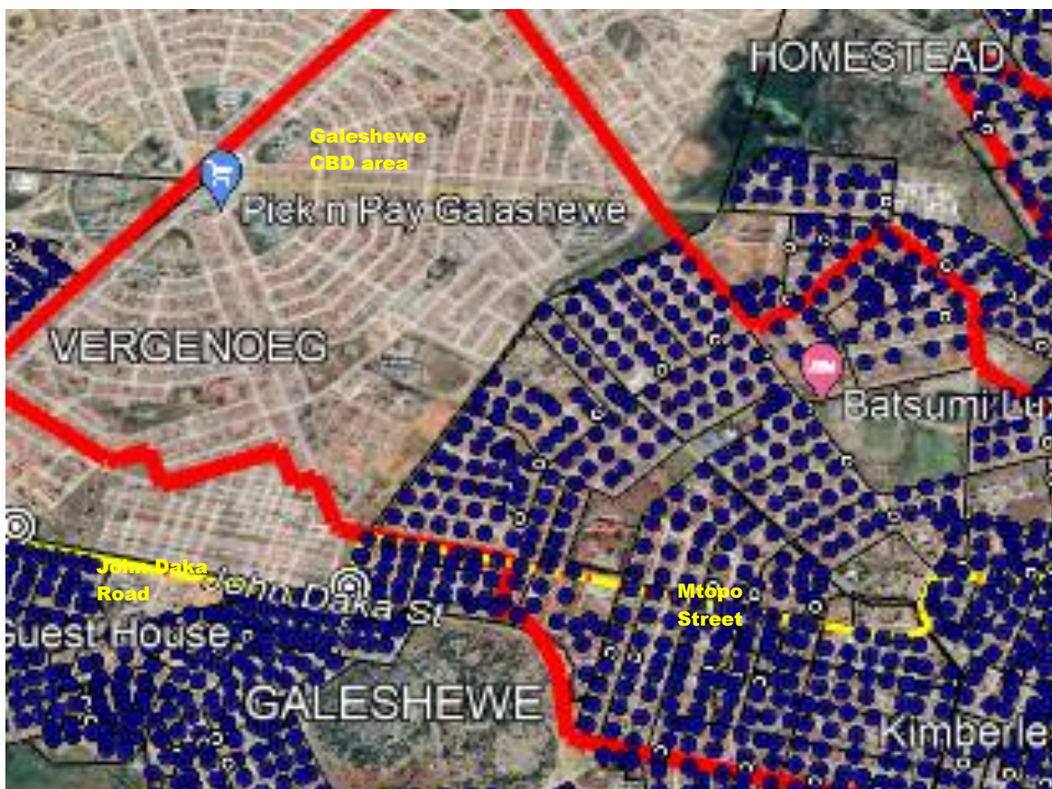
Figure 24: Section 4 of Route 1 (Galeshewe): Yellow line indicates the underground main line and the blue dots the position of the poles for the aerial fibre. The red lines show the boundary of the area older than 60 years.
