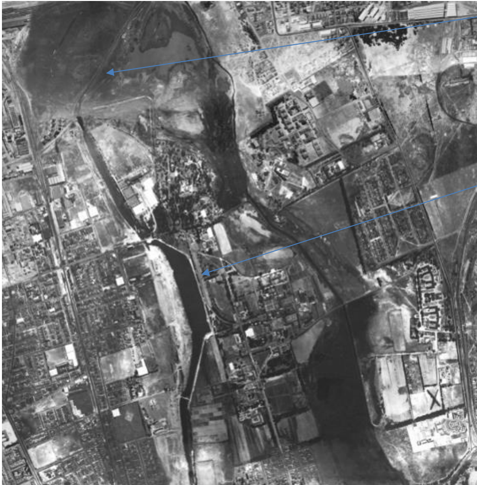
Fig 7.8. 1945 Aerial photograph showing original course of the Liesbeek River (arrowed) the wide water body in front of the Valkenburg Hospital and the continuing canalisation of the Black and Liesbeek Rivers.
