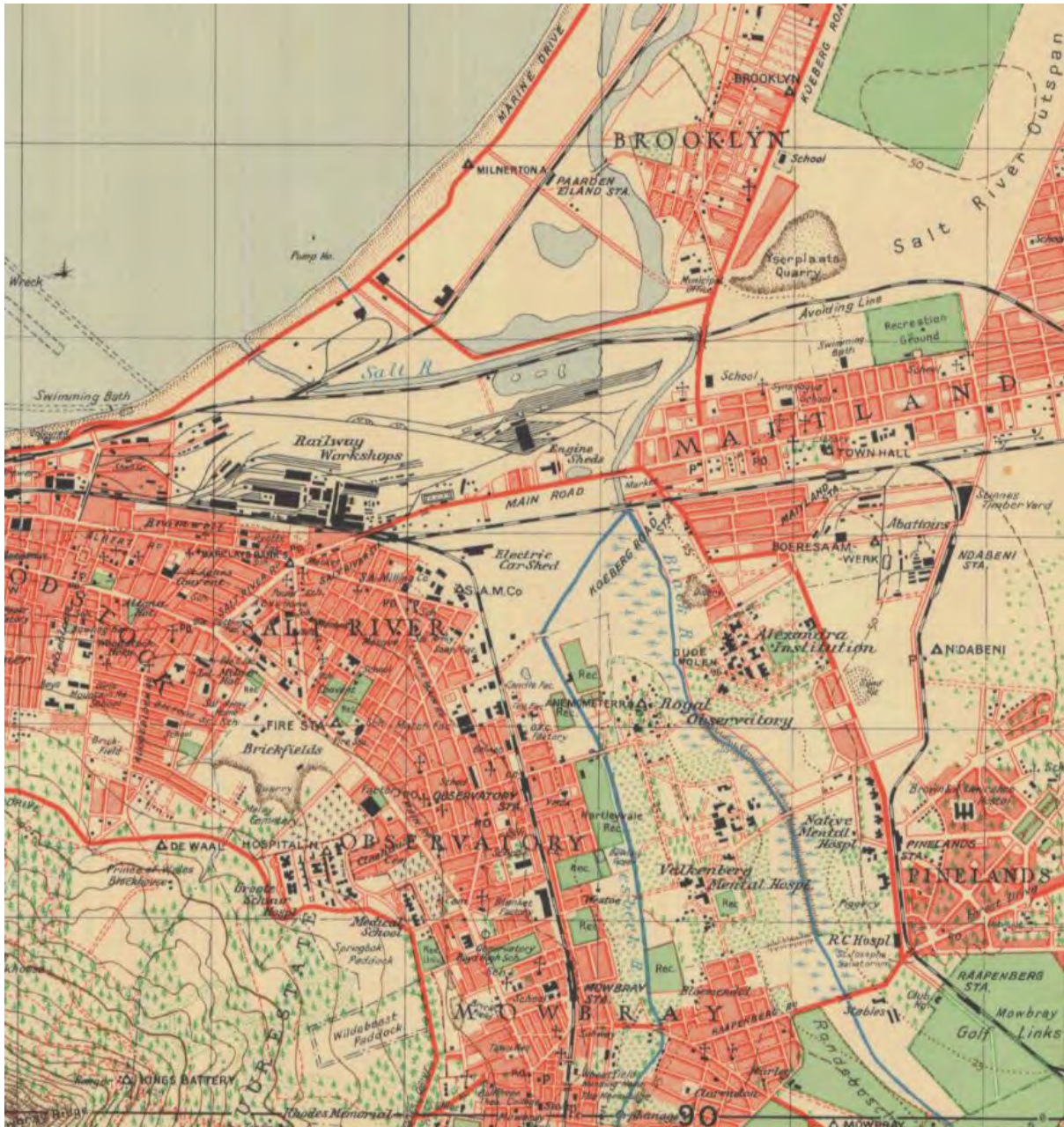
Figure 2. An excerpt from 1:25 000 map of 1935 (Chief Directorate: Surveys and Mapping) which reveals that by that time a large portion of the Salt River estuary had been filled for railway development and the river diverted. Furthermore indications are that the Liesbeek had been straightened for a significant amount of its length. It is of interest to note that the Maitland Outspan became Ysterplaats airforce base.
