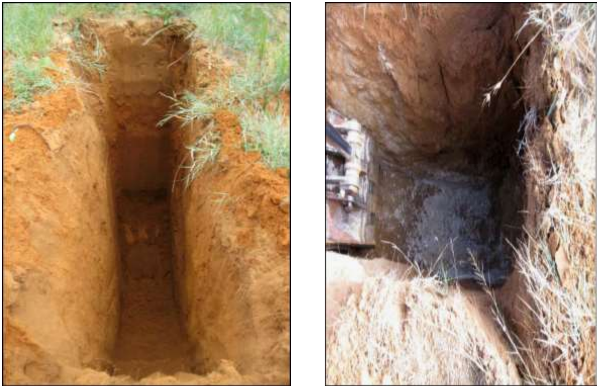
Fig. 3. Field photos from the geotechnical report for the Droogfontein development site showing deep orange-hued Kalahari sands (LHS) with pale calcrete at depths of c. 2.5m in some trial pits (Mainstream Renewable Power, 2011).
