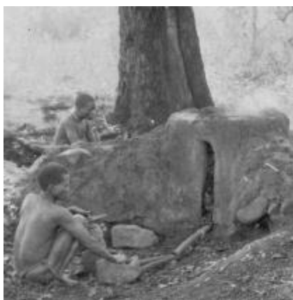
Fig. 09. In his Diary Gros wrote; '... Makaties 16 iron founder, Iron Mountain, low country east of Spelonken. The ore which is gathered in the vicinity is smelted twice in a furnace of common clay, charcoal being used. Three chinks in the sides, and a blower at each, supply the oxygen by means of a skin bag held in each hand and worked alternately up and down with great rapidity, the bags being filled in the upward motion by relaxing the opening held in the hand. On being removed from the furnace the incandescent mass is beaten hard and fast between stones, and taken to the village, where it is manufactured into utensils, which becomes currency. (Picture by Gros in 1885.)
