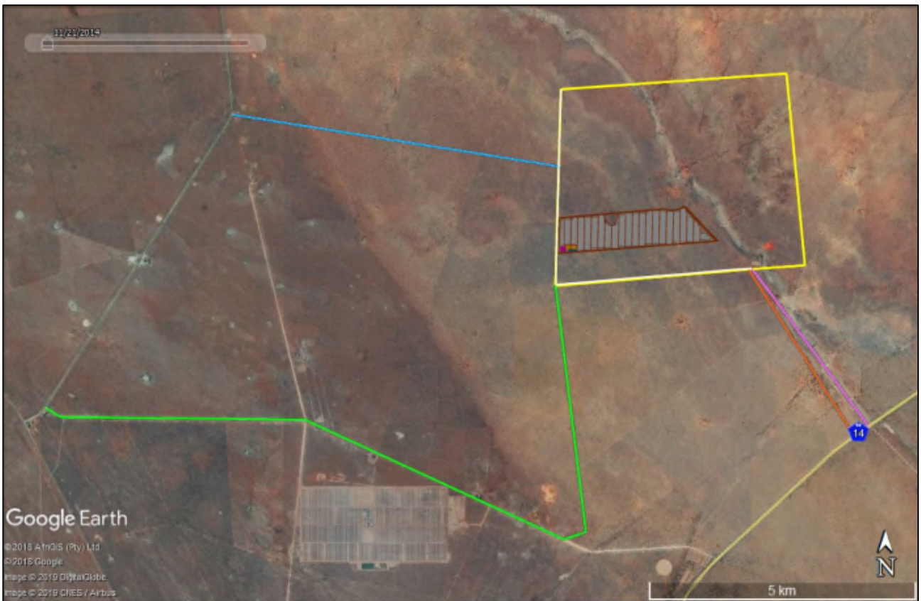
Figure 2: Aerial view of the broader study area showing the project site (yellow polygon), proposed HSD3 development area (grey hatched area), four access road alternatives (See Fig. 1 for labels) and the proposed perimeter access road (white line along western and southern margins of the site).
