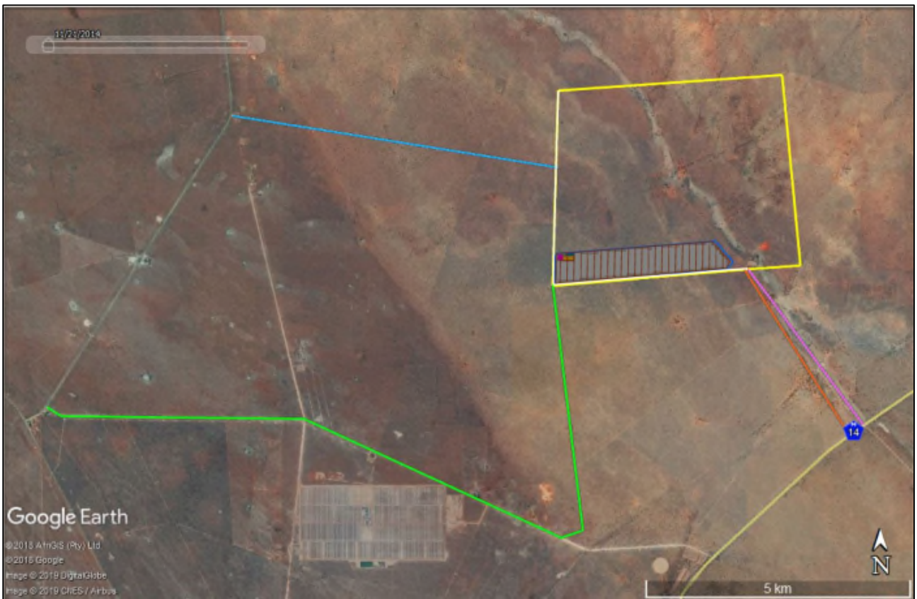
Figure 2: Aerial view of the broader study area showing the project site (yellow polygon), proposed HSD4 development area (grey hatched area), four access road alternatives (See Fig. 1 for labels) and the proposed perimeter access road (white line along western and southern margins of the site).
