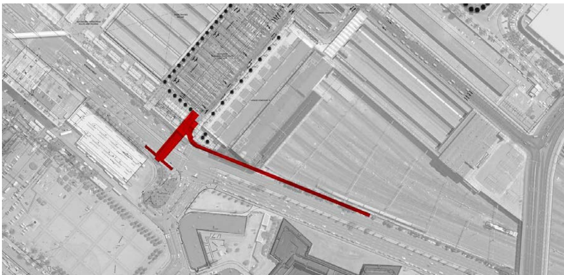
FIGURE 1C: Inner City Transportation Hub current proposal: Location of Project A: A pedestrian bridge replacing the current one on the same site; and Project B: the vehicular ramp and setback of the building façade, which remains unchanged.
