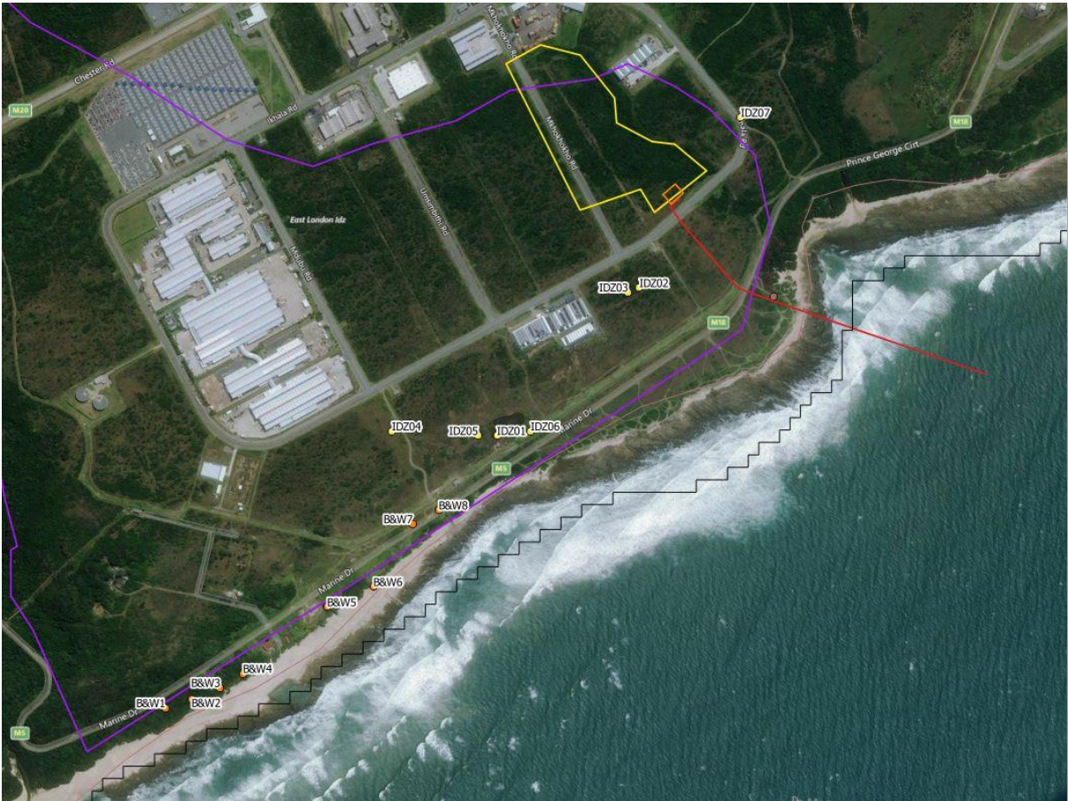
Figure 1: The IOX cable landfall, re-aligned terrestrial cable route (red line) and beach manhole (orange polygon) and surrounding area. The items marked as B&W and IDZ are archaeological sites found during previous surveys of the area which are discussed in Section 6 below
