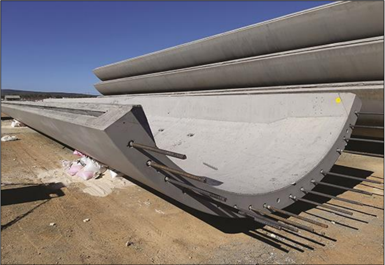
Figure 3: Proposed precast concrete section of wind turbine mast.
