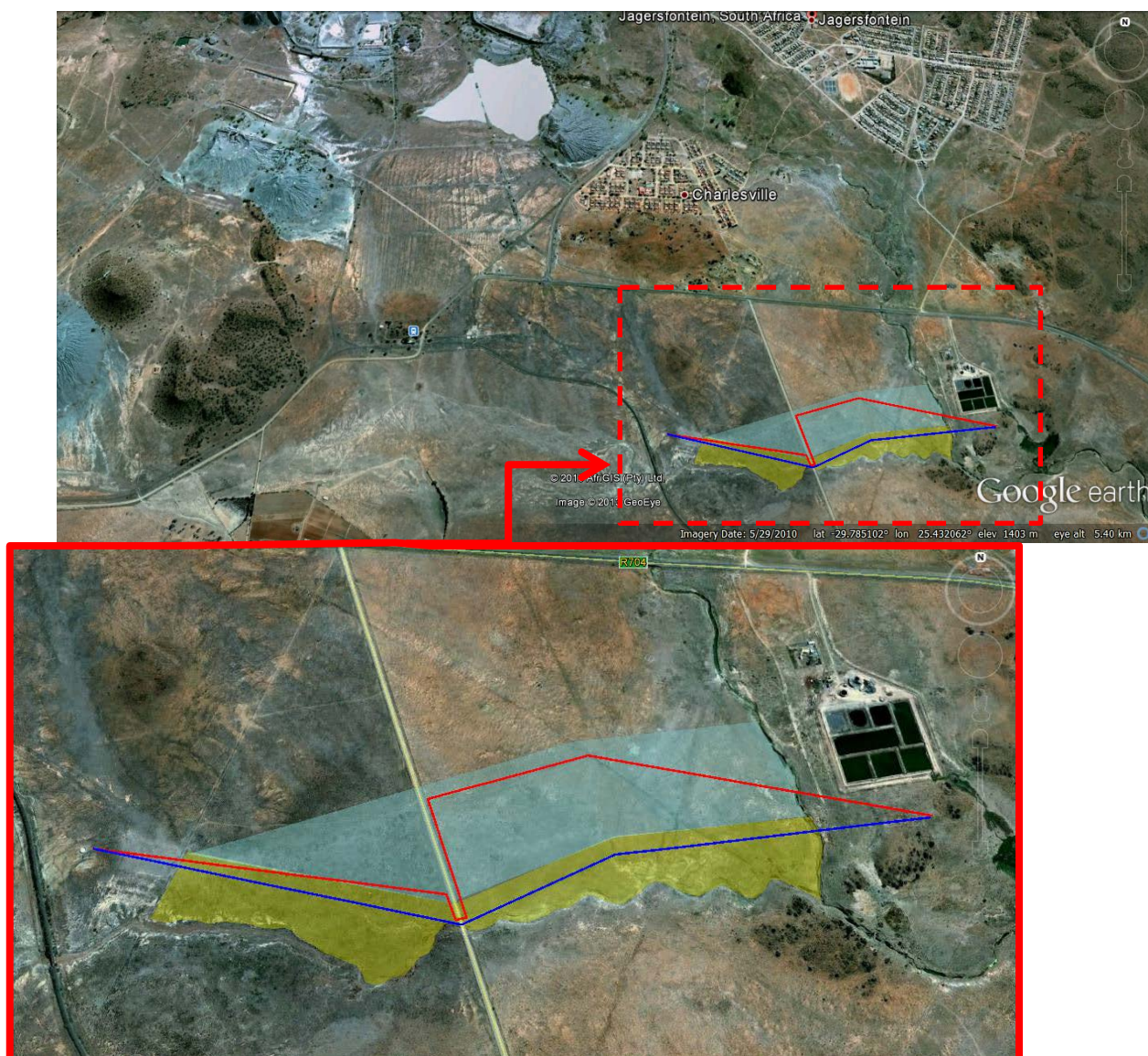
Figure 12: Original surveyed area blocked in yellow (blue line is the position of the original proposed pipeline). Extended survey area blocked in blue; red line is proposed alternative route for the new pipeline
