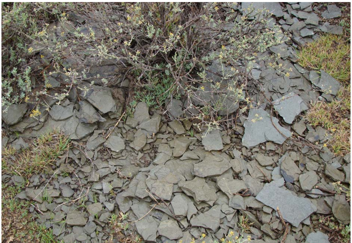
Figure 16: A shale outcrop in an advanced state of disintegration
