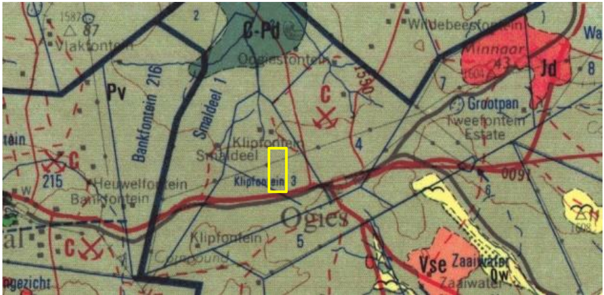
Figure 2: Geological map of the area around the Farm Klipfontein. The location of the proposed WTP pipelines is indicated within the yellow rectangle. Abbreviations of the rock types: C-Pd = Dwyka Group; Pv = Vryheid Formation; Jd = Jurassic dykes Map enlarged from the Geological Survey 1: 250 000 map 2628 East Rand ERPM.
