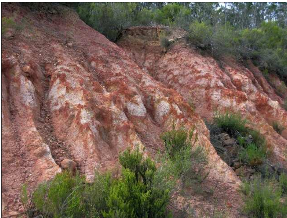
Fig. 26. Thick, sparsely gravelly, semi-consolidated sandstones of possible alluvial origin showing prominent mottling by reddish-brown ferruginous minerals, R62 roads cutting (Loc. 038).
