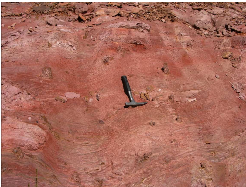
Fig. 18. Close-up of weathered, ferruginised Gydo Formation in R62 road cutting at Loc. 025 (Hammer = 27 cm). Note prominent-weathering lenticles or blobs of secondary minerals.
