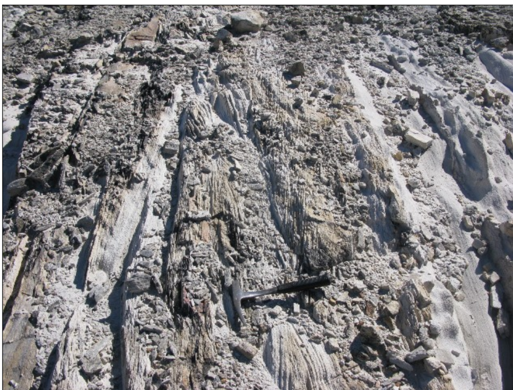
Fig. 11. Borrow pit exposure of highly weathered, interbedded sandstone / mudrock succession along the Suuranysberg Pass (Loc. 029) (Hammer = 27 cm). These rocks belong to either the upper Cederberg Formation (Disa Member) or the overlying Goudini Formation.
