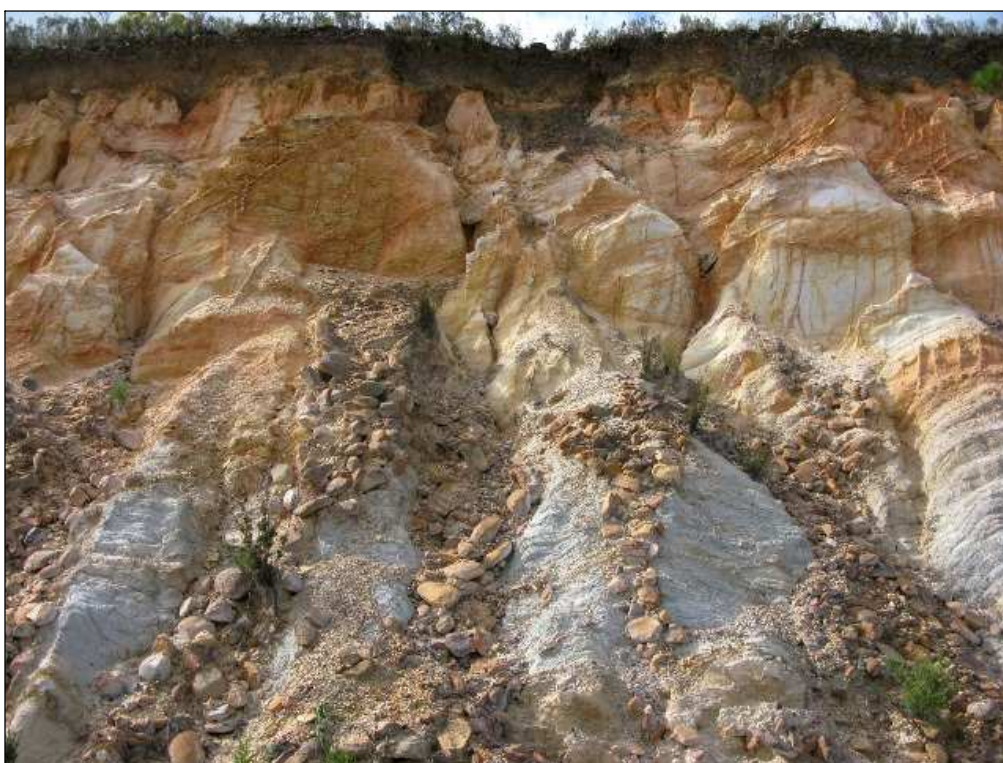
Fig. 15. Deeply weathered arenites of the Baviaanskloof Formation along the R62 (Loc. 037). Note irregular erosional contact with the overlying gravelly soils.
