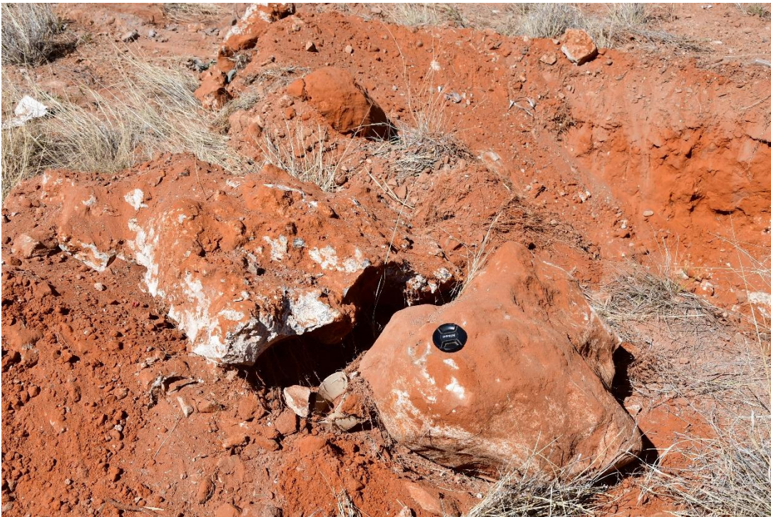
Figure 13. Large nodules of calcrete removed from Trench 5, camera lens cap for scale.
