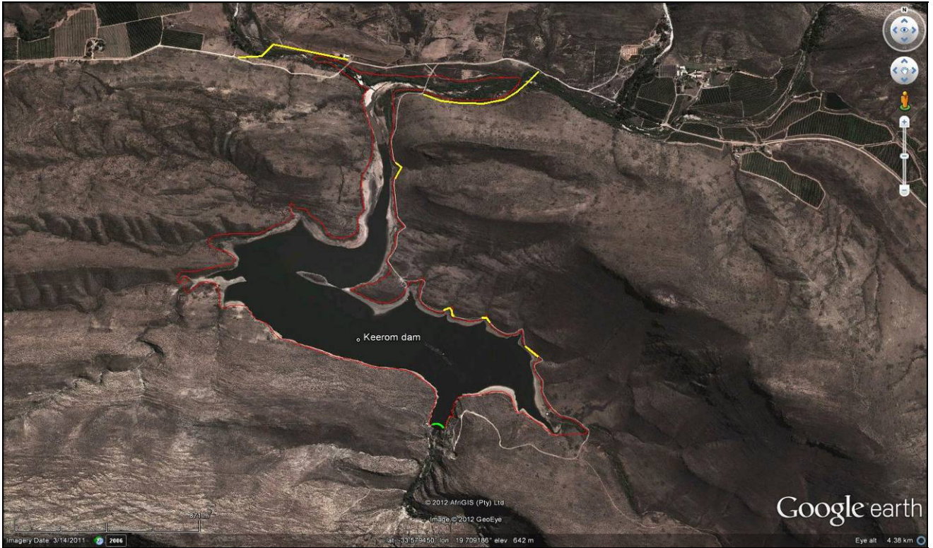
Figure 2: Detail showing the existing dam wall (green) and increased FSL (red). Road re-alignments (yellow).
