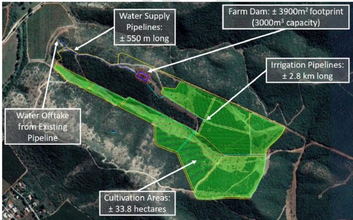
Map 3. The layout of the development on Portion 2 of the farm Keurkloof No. 56 (images courtesy Habitat Link Consulting).
