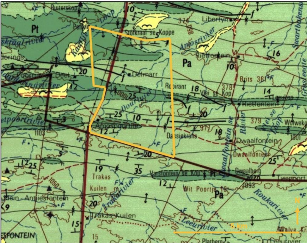
Figure 19: Extract from 1: 250 000 geology sheet 3222 Beaufort West showing the boundaries of the Kraaltjies WEF project area to the south of Beaufort West (orange polygon). Note numerous W-E trending fold axes occur in the region which falls within the northern margins of the Cape Fold Belt. Pa (pale green) = Abrahamskraal Formation (Adelaide Subgroup, Lower Beaufort Group). Pt (dark green) = Poortjie Member of the Teekloof Formation (Adelaide Subgroup, Lower Beaufort Group). Yellow = Late Caenozoic / Quaternary superficial sediments, including alluvium (flying bird symbol), as well as unmapped sheet wash, colluvium, soils, locally cemented by pedocretes such as calcrete. To the west of the N12 and outside the WEF / Grid Connection Infrastructure project area diamond symbols indicate fossil localities within the Tapinocephalus Assemblage Zone. Triangles indicate fossils within the Pristerognathus Assemblage Zone (N.B. This fossil biozone data is now outdated and the fossils concerned have probably been collected).
