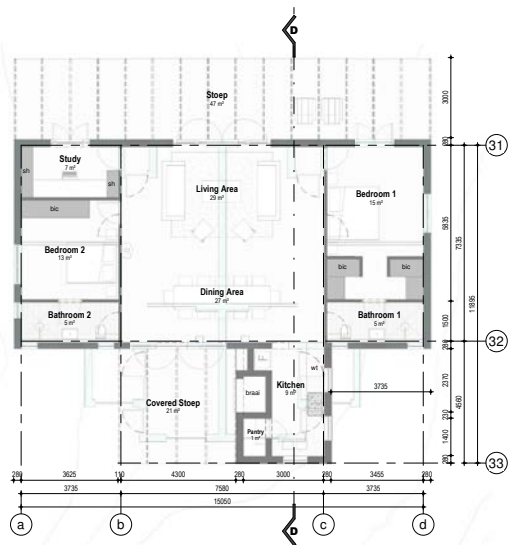
FFL_Ground Floor - Derek Cottage SCALE 1:100
