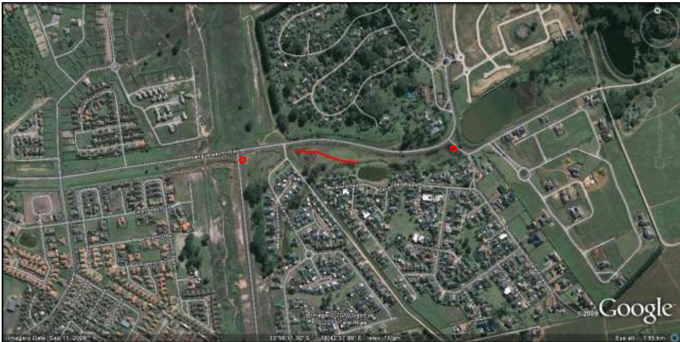
Figure 2: Aerial photograph (from Google Earth) of the study area showing the location of the proposed berm (red line). Other minor remedial measures will occur at the two red circles.
