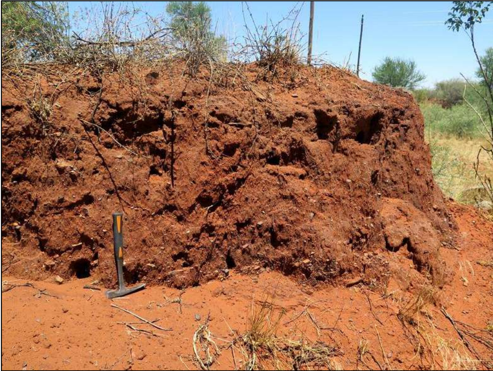
Figure 45. Rusty-brown alluvial sands with dispersed fine gravels exposed in a borrow pit near Wrenchville (Hammer = 30 cm) (Loc. 240).
