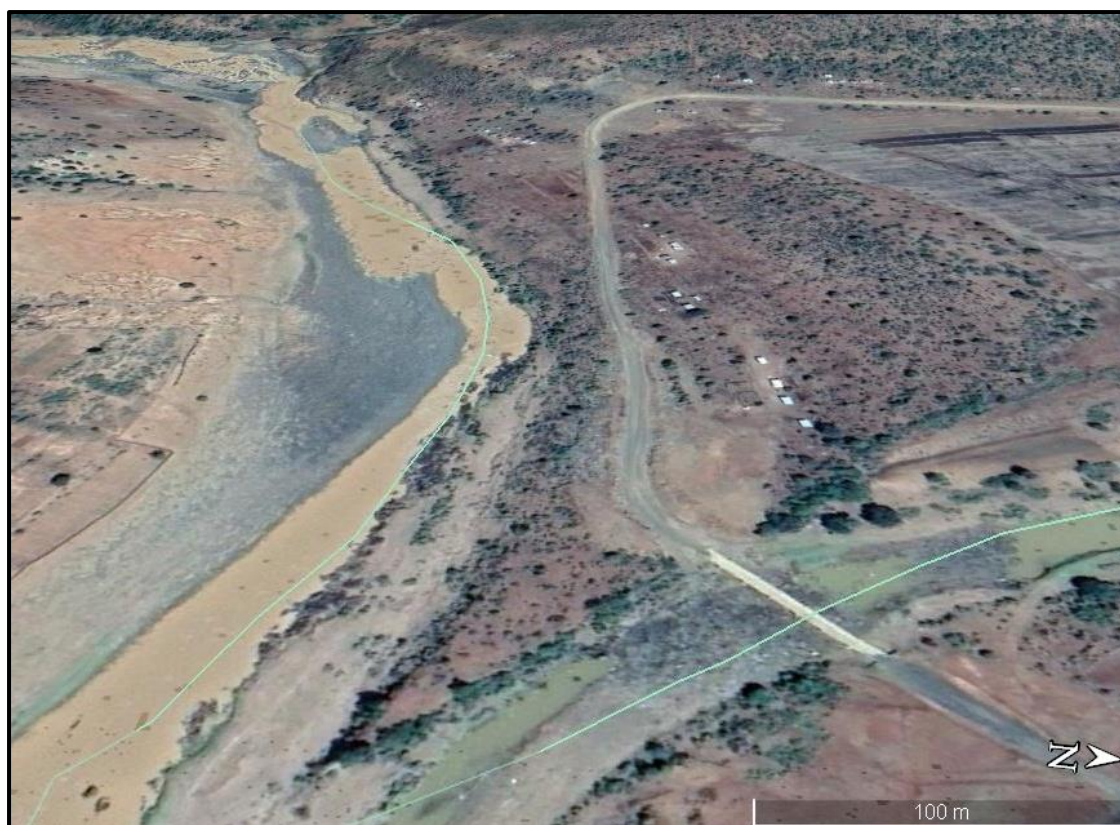
Figure 2: Satellite image showing the starting point of the proposed road, at the bridge crossing. This section of the road is already well established and is built on top of dolerite and Quaternary deposits. North is to the right of the image. Modified Google Earth image, AfriGIS 2019
