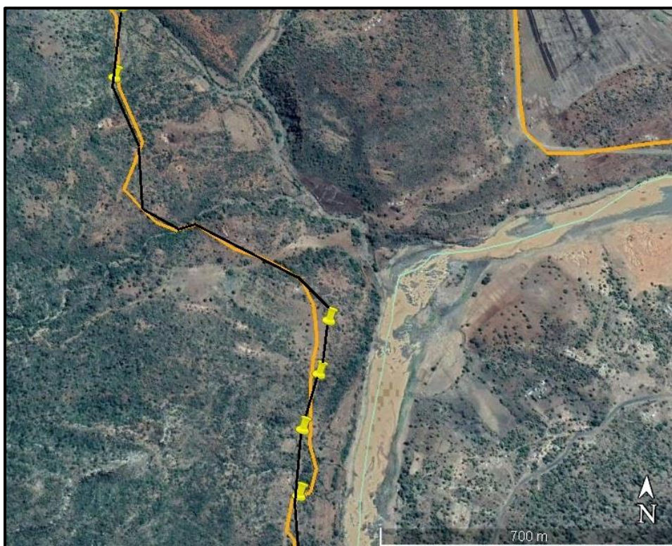
Figure 12: Satellite image showing a suggested alternative route for the proposed road, indicated in black. This option tries to avoid vegetated areas and to rather stick to existing paths and open patches of ground
