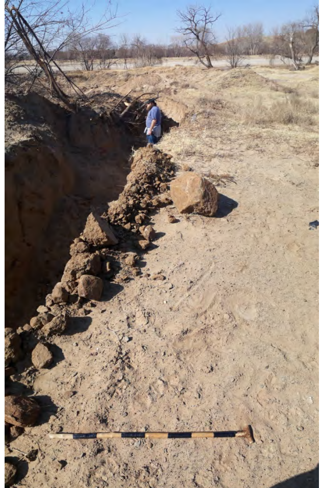
Figure 14. Exposed, degraded terrain resulting from previous sand mining activities (left) and current construction activities (right), showing well-developed alluvial sand packages of up to 4m in depth, exposed within the overbank sediments within the proposed mining area. Scale 1 = 10 cm.
