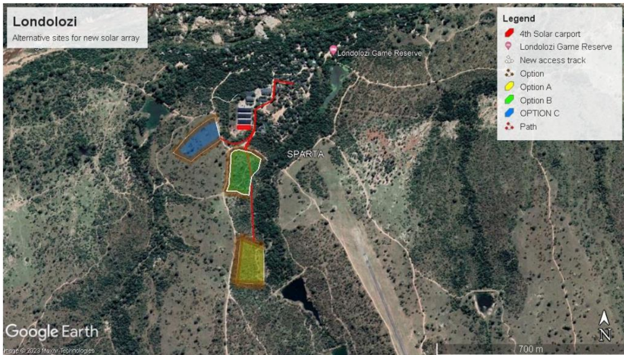
Figure 2: The location of the three alternative sites for the proposed solar array and transmission infrastructure.
