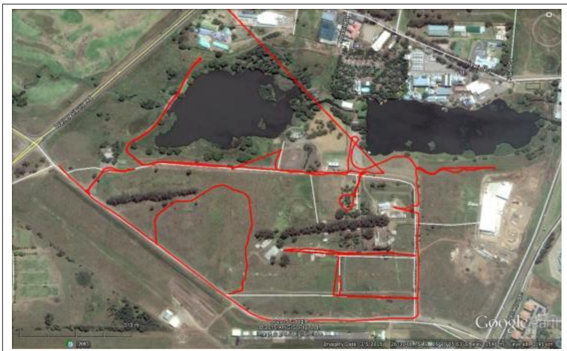
Figure 1- The main track according to which the survey was conducted was recorded with a GPS instrument which was mounted in a vehicle. Pedestrian surveys were conducted from the main track (above).
