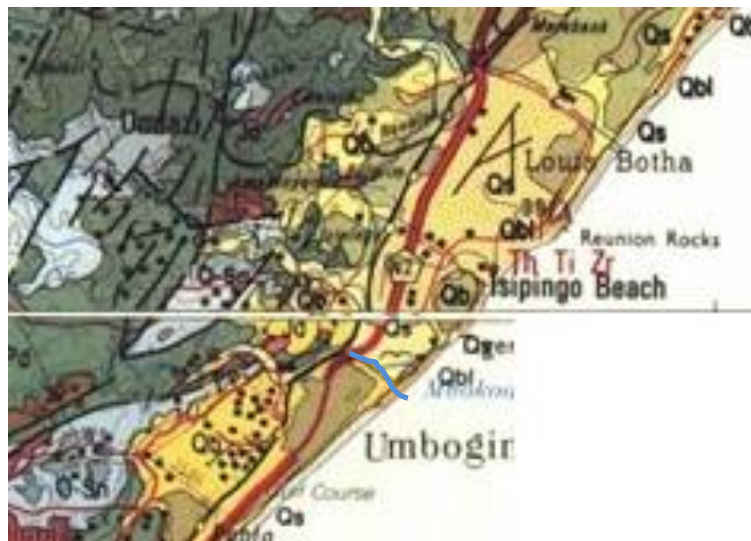
Figure 2: Geological map of the area around Isipingo and Umbogintwini. The proposed culvert is indicated by the blue line. Abbreviations of the rock types are: Qs = alluvium or beach sand (dotted); Qb = Umkwelane Formation. Top map enlarged from the Geological Survey 1: 250 000 map 2930 Durban, and bottom map 3030 Port Shepstone.
