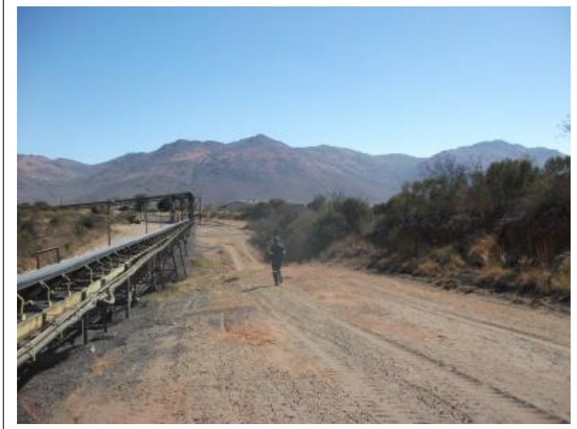
Figure 4- The existing Slag Overland Conveyer will be re-aligned from the Smelting Plant to the Slag Dump (above).
