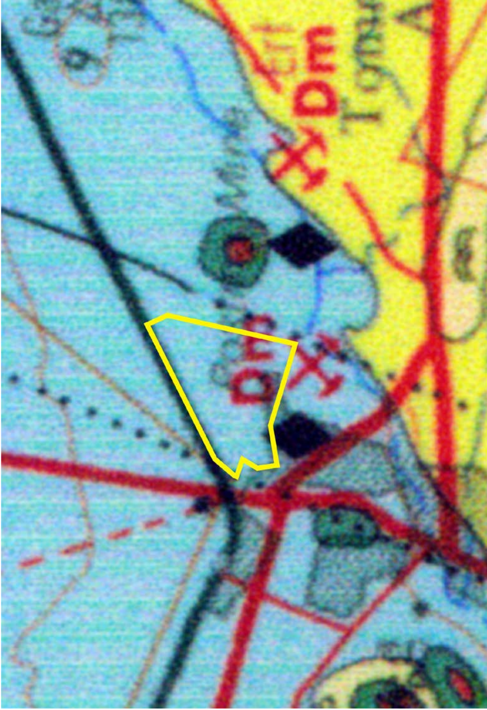
Figure 4. According to the 1:250 000 scale geological map 2822 Postmasburg, the proposed development footprint is underlain by palaeontologically significant carbonate rocks of the ~2.5 Ga old Cambellrand Subgroup (Vgl, Ghaap Group, Transvaal Supergroup).
