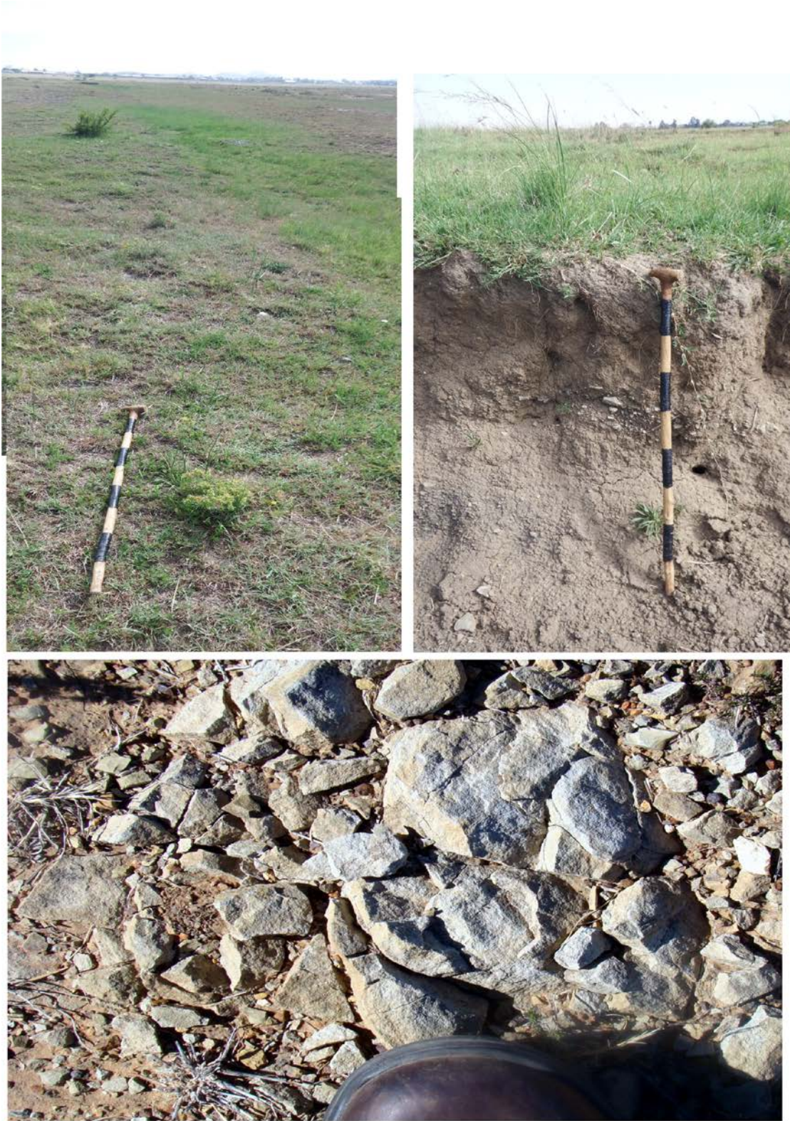
Figure 6. Superficially degraded alluvial and residual soil deposits top (left & right), unconformably overlain by fine to medium-grained Katberg Formation sandstones (below).
