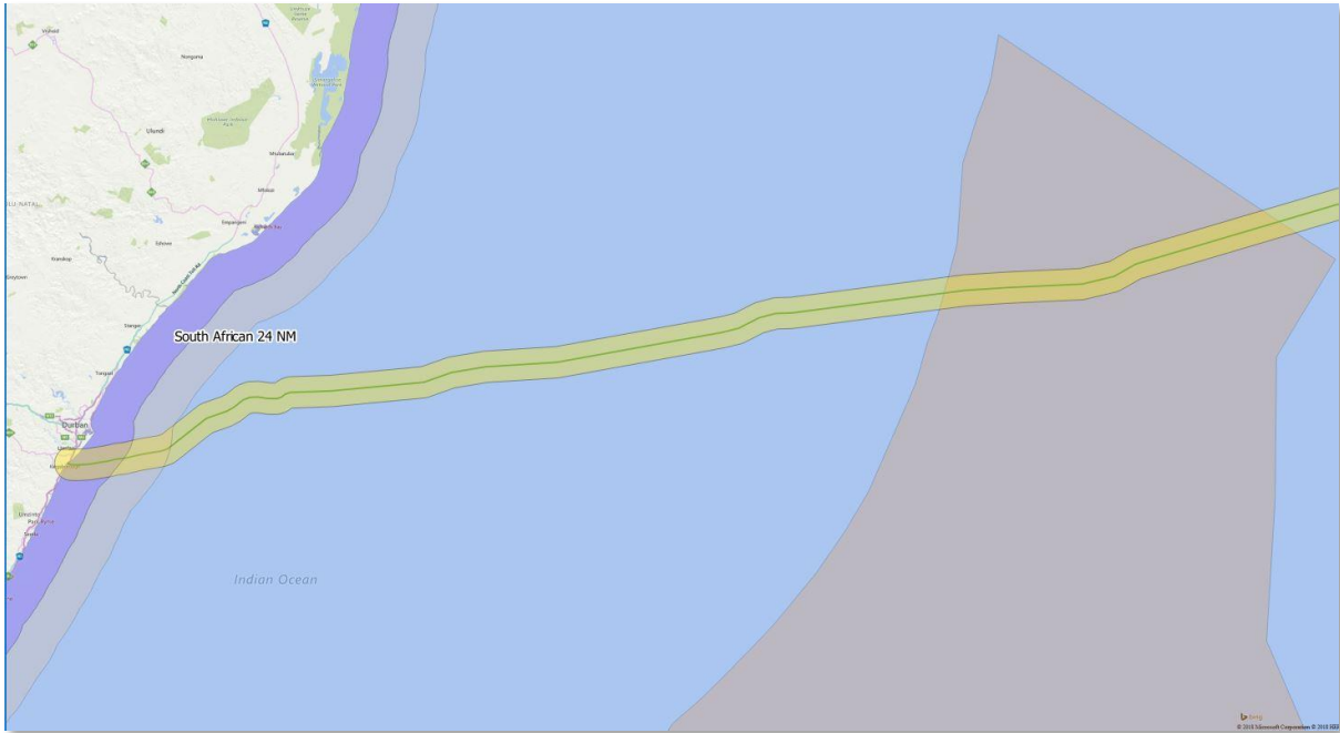
Figure 1: Route of the proposed METISS subsea cable from the outer edge of the South African continental shelf to the landfall at Amanzimtoti on the KZN coast.
