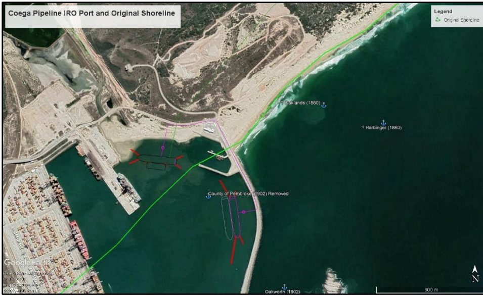
Figure 1: Port of Ngqura original shoreline, County of Pembroke position and proposed pipelines
