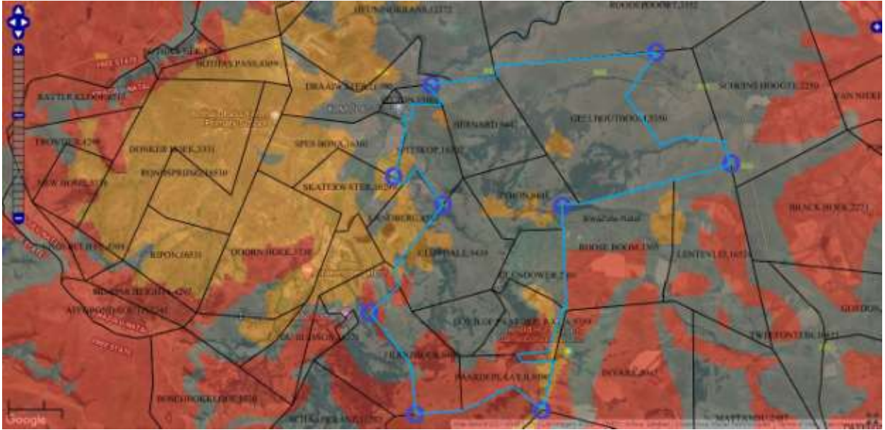
Figure 6: Palaeosensitivity of rocks in the Mulilo Newcastle WEF footprint (blue outline). Most of the area is dolerite (grey) and of no concern however the thickness of the dolerite is unknown.
